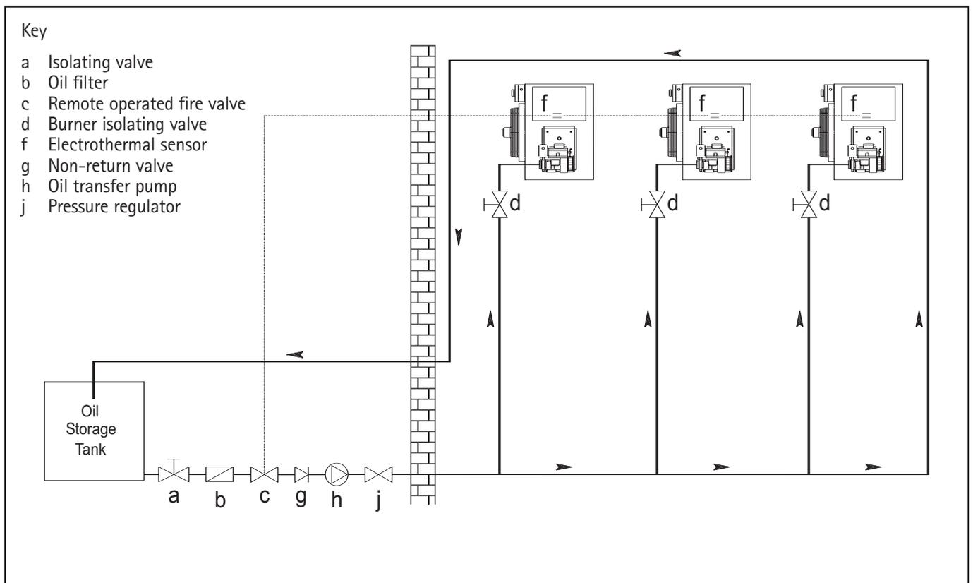
Fig 5 Single heater installation with oil lifter
