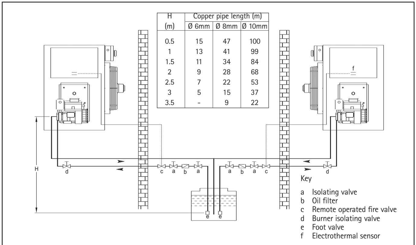
Fig 4 Multiple heater installation with oil transfer pump (two-pipe system shown)
